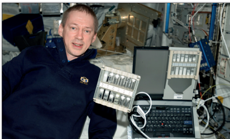
▼ FIG. 2: Astronaut Frank de Winne with the foam cells in the ISS; a cell rack is free floating in the centre of the picture and a second rack is placed in front of a computer screen for backlight illumination during video recording. Image courtesy of ESA.
