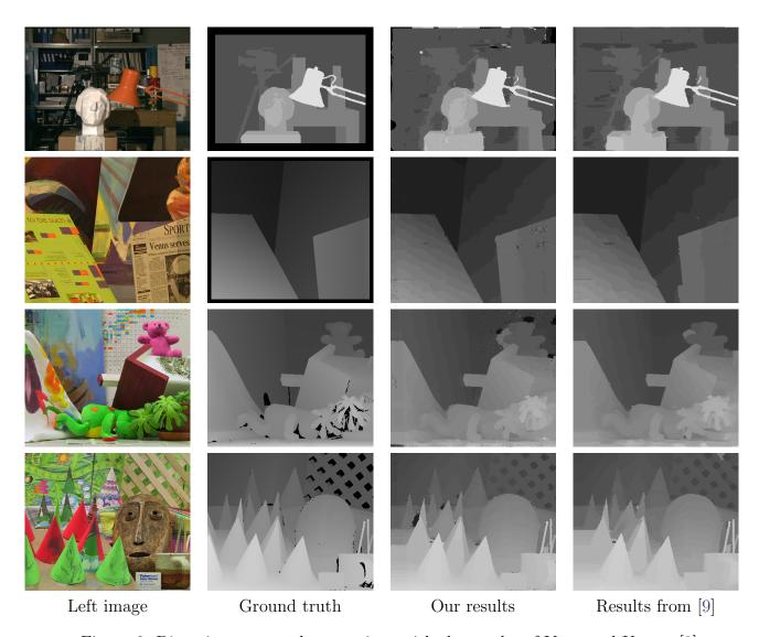
Figure 6: Disparity maps and comparison with the results of Yoon and Kweon [9].
