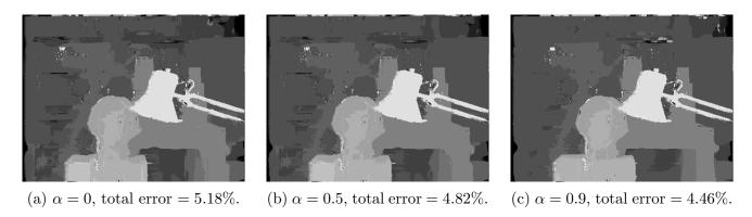
Figure 5: Disparity maps for Tsukuba for different values of  $\alpha$  without the post-processing step.
