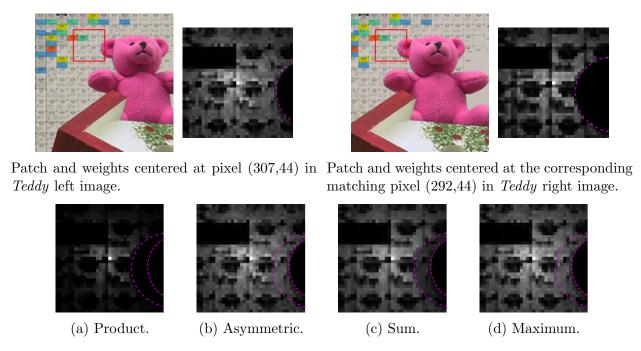
Figure 11: Example of the resulting weights for the matching cost computation of two patches using different combinations of weights.
