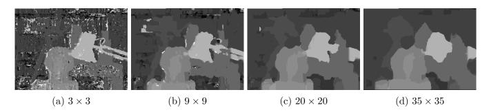
Figure 2: Resulting disparity maps for *Tsukuba* obtained with a simple block-matching method (using SAD, sum of absolute differences, for patch similarity) for several patch sizes. The visible dilation of foreground shapes appearing with the increase of the patch size is the fattening phenomenon.
