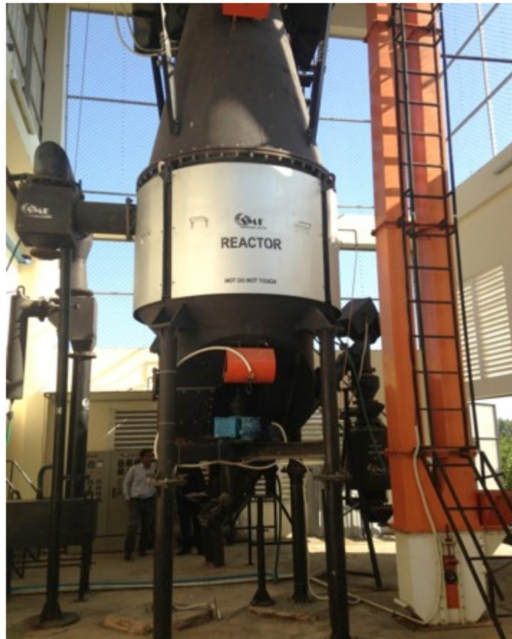
**Figure 3:** 600kW Gasifier at Golden Daun Keo rice mill, Battambang, Cambodia, 2014-12-20
