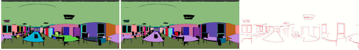
Figure 2: Segmentation by region growing (left), plane fusion (middle) and line segments selected for ghosts generation.
