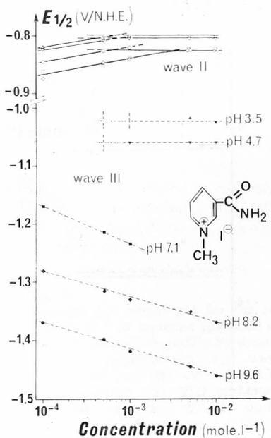
Fig. 7. Effect of the concentration of  $N_1$  methyl nicotinamide iodide on its reduction waves position (—) wave II and (---) wave III. pH and buffer conditions: ( $\blacktriangle$ ) 3.56 formate, ( $\blacktriangledown$ ) 4.68 acetate, ( $\blacksquare$ ) 7.15 imidazole, ( $\blacklozenge$ ) 8.25 tris and ( $\bullet$ ) 9.57 borate.
