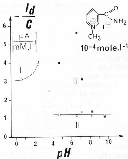
Fig. 5. Diagram  $I_d/c$  versus pH for the reduction of  $10^{-4} M$  aqueous solutions of N<sub>1</sub> methyl nicotinamide iodide by drop-time controlled polarography: (○) wave I, (●) wave I' and (■) wave III. Conditions: capillary 10, 35.0 cm mercury, controlled drop-time 0.5 s, potential sweep rate 0.25 V/min,  $m = 0.86 \pm 0.03$  mg s<sup>-1</sup>.
