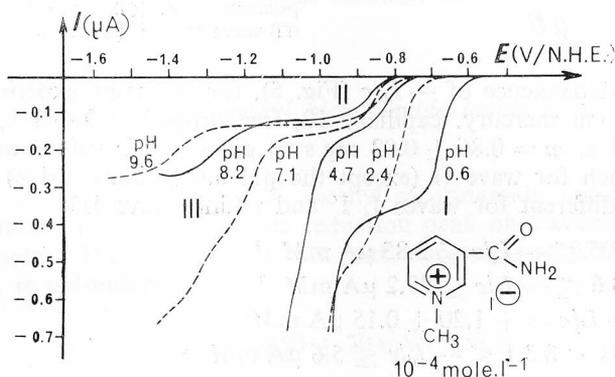
Fig. 3. Reduction of  $10^{-4}$  M aqueous solutions of  $N_1$  methyl nicotinamide iodide by drop-time controlled polarography: pH 0.56 (HCl), 2.41 (glycine), 4.68 (acetate), 7.15 (imidazole), 8.25 (tris) and 9.57 (borate).
