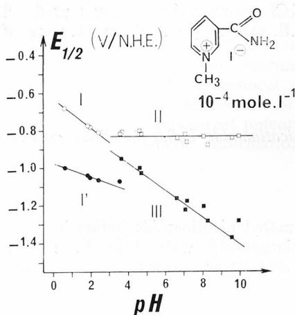
Fig. 4. Diagram  $E_{1/2}$  versus pH for the reduction of  $10^{-4} M$  aqueous solutions of N<sub>1</sub> methyl nicotinamide iodide by drop-time controlled polarography: (○) wave I, (●) wave I', (□) wave II and (■) wave III.
