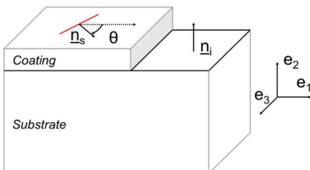
Figure 7 - Virtual surface crack and normal vector illustration
