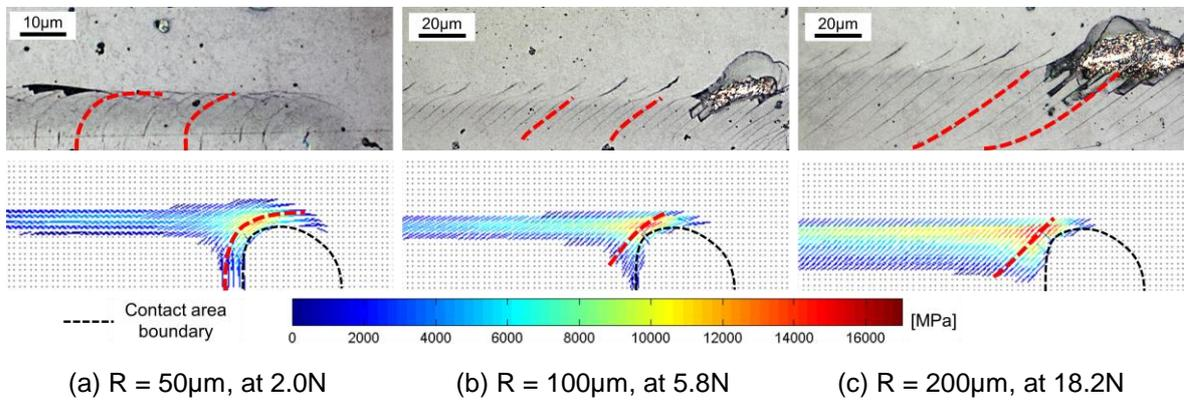
Figure 6 – Surface cracks before failure (top) and first principal stress at the critical load (bottom)
