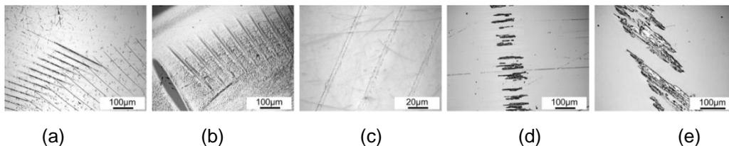
Figure 4 - Scratch network examples from a cam-tappet system [3]
