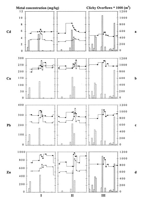
*Figure 6.* Metals concentration variations in SS sampled at Suresnes ( $\otimes$ ) and Chatou ( $\blacksquare$ ) from 17/6/92 to 15/7/92 (I), from 16/8/92 to 13/9/92 (II) and from 8/9/93 to 6/10/93 (III), and volume of Clichy overflows ( $\Box$ ): (a) Cd, (b) Cu, (c) Pd and (d) Zn.
