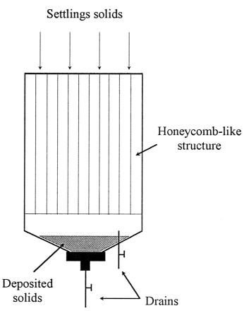
Figure 2. Suspended solid trap.
