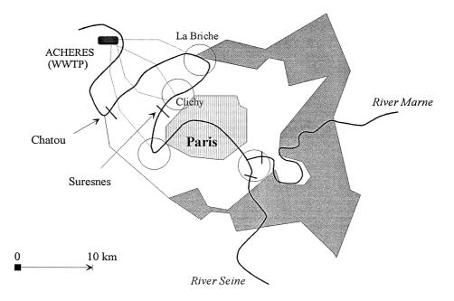
*Figure 1.* Map of Paris conurbation. The grayed area is drained by a separate sewer system while the centrale white area is drained by a combined system. Circles figure the areas where major combined sewer overflow occur. Small perpendicular bars figure the navigation dams where traps were deployed.
