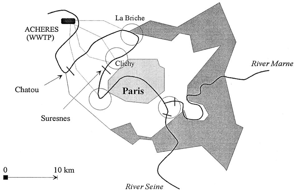
Figure 1. Map of Paris conurbation. The grayed area is drained by a separate sewer system while the centrale white area is drained by a combined system. Circles figure the areas where major combined sewer overflow occur. Small perpendicular bars figure the navigation dams where traps were deployed.
