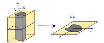
Figure 3: Representative unit cell under generalized plane strain conditions.
