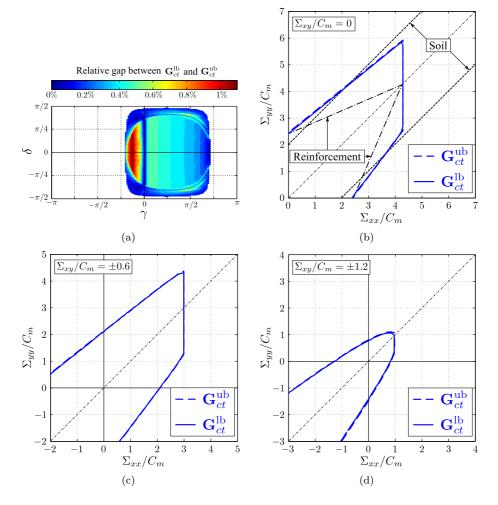
Figure 14: Bounds of the macroscopic strength criterion of a cross trench reinforced soil with  $\Sigma_{xy}/C_m$  fixed.
