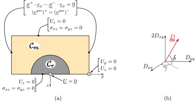
Figure 8: Boundary conditions for the determination of the plane strain macroscopic strength criterion (a) and macroscopic strain rate directions (b).
