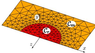
Figure 9: Finite element model adopted for obtaining the numerical lower and upper bounds.
