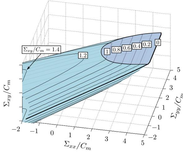
Figure 13: Upper bound of the macroscopic strength domain of a cross trench reinforced soil.
