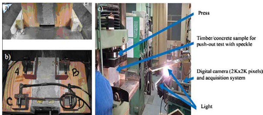
Fig. 7. (a) Sample position under the compressive tool with wedges to block horizontal displacement. (b) Push-out instrumented sample and (c) Optical set-up for DIC measurements during mechanical tests.
