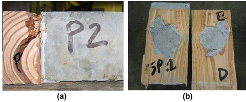
Fig. 8. Failure mode within wood ring (left) (a) and Failure mode disturbance due to a knot (right) (b).
