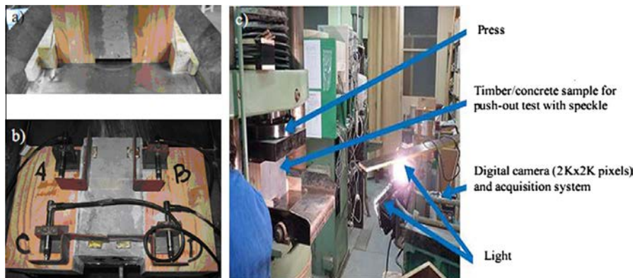
Fig. 7. (a) Sample position under the compressive tool with wedges to block horizontal displacement. (b) Push-out instrumented sample and (c) Optical set-up for DIC measurements during mechanical tests.
