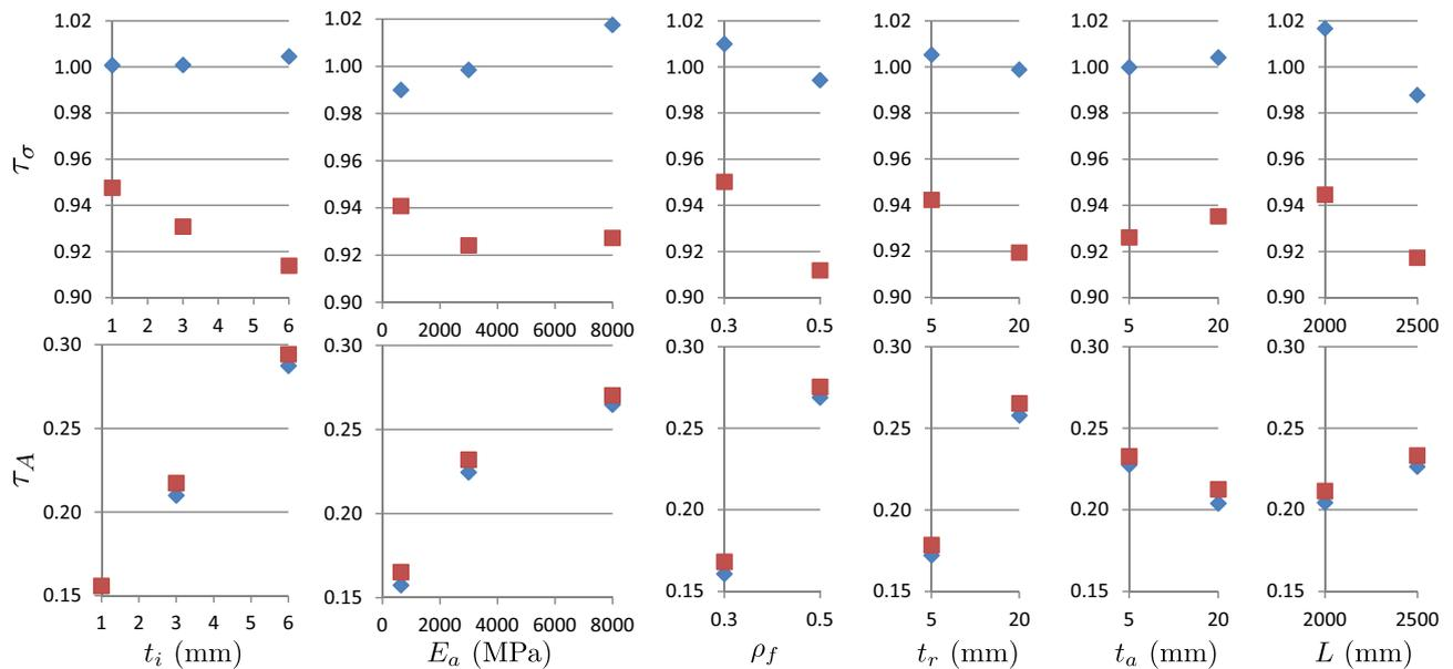
Fig. 11.: Sensitivity analysis for the Triple Skew Diamond factorial experiment. Blue markers are for the uni-axial strain and brown markers for the uni-axial traction load cases.
