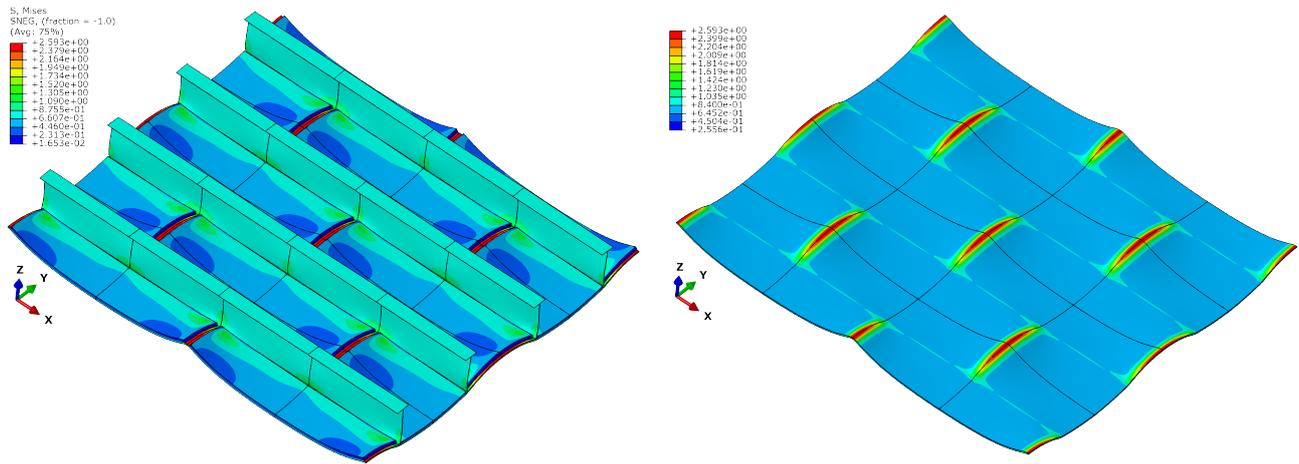
Fig. 7.: Global view of the reinforced hull with rectangular pads. The hull is under uni-axial strain in Direction x and the contour plot is the stress rate. 4 unit-cells are displayed.
