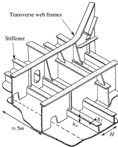
Fig. 3.: Structural detail of the FPSO unit bottom
