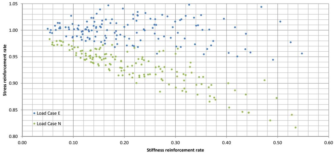
Fig. 10.: Stress reinforcement rate vs. Stiffness reinforcement rate for the Triple Skew Diamond factorial experiment
