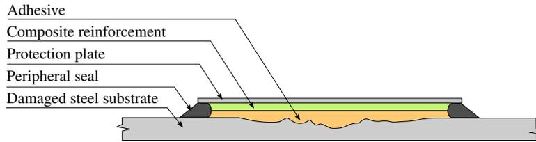
Fig. 1.: Typical cross section of a single pad
