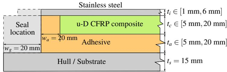
Fig. 5.: Cross section modeled with FE
