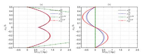
**Fig. 10** Normalized shear distribution in both directions at  $x_1=0$  for a  $[-30^\circ,30^\circ]$  laminate, L/h=4, a)  $\sigma_{13}$  b)  $\sigma_{23}$ .
