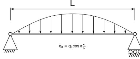
**Fig. 2** Pagano's cylindrical bending configuration
