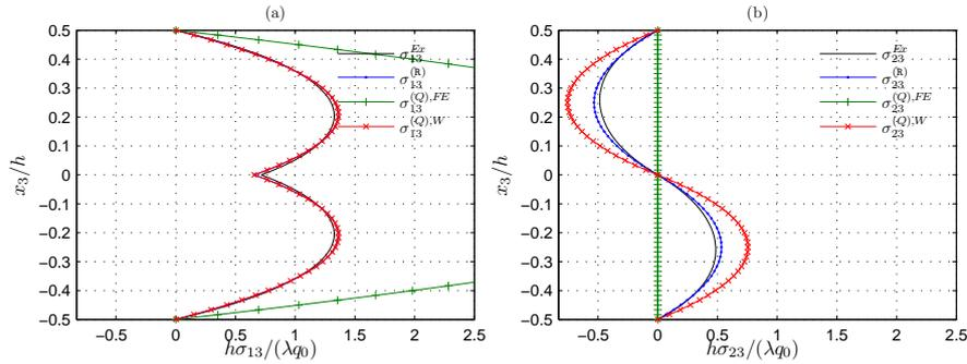
**Fig. 10** Normalized shear distribution in both directions at  $x_1 = 0$  for a  $[-30^\circ, 30^\circ]$  laminate,  $L/h = 4$ , a)  $\sigma_{13}$  b)  $\sigma_{23}$ .
