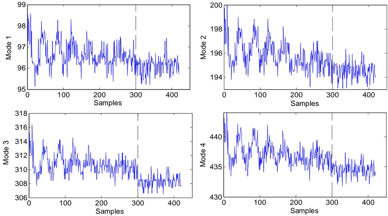
Figure 3: Evolution of the natural frequencies [Hz] throughout the tests carried out on the quasi-stationary system: damage introduced by saw-cut after the 300<sup>th</sup> sample (dashed vertical line).
