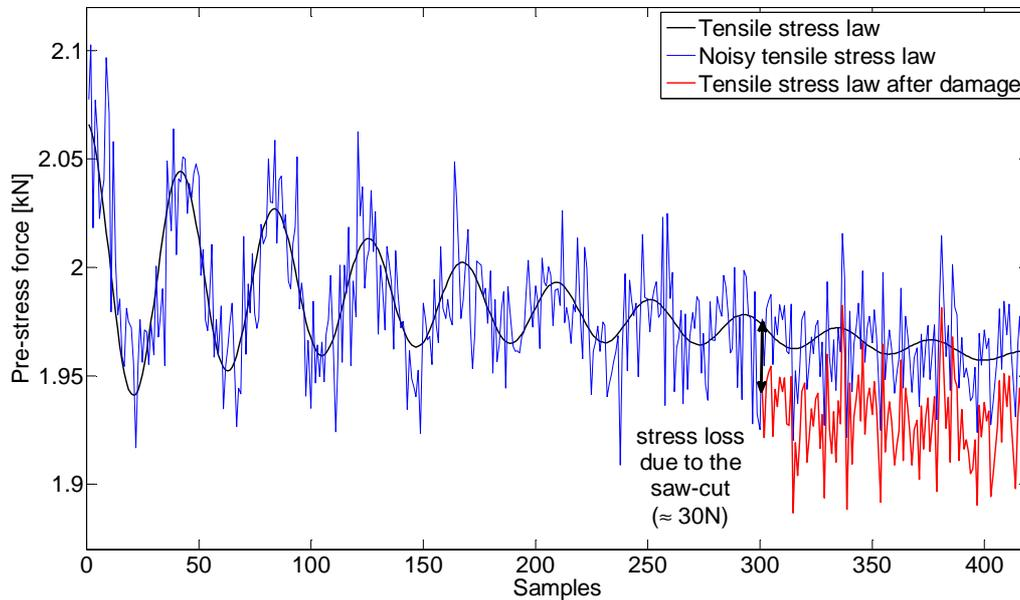
Figure 2: Pre-stress force applied to the beam.
