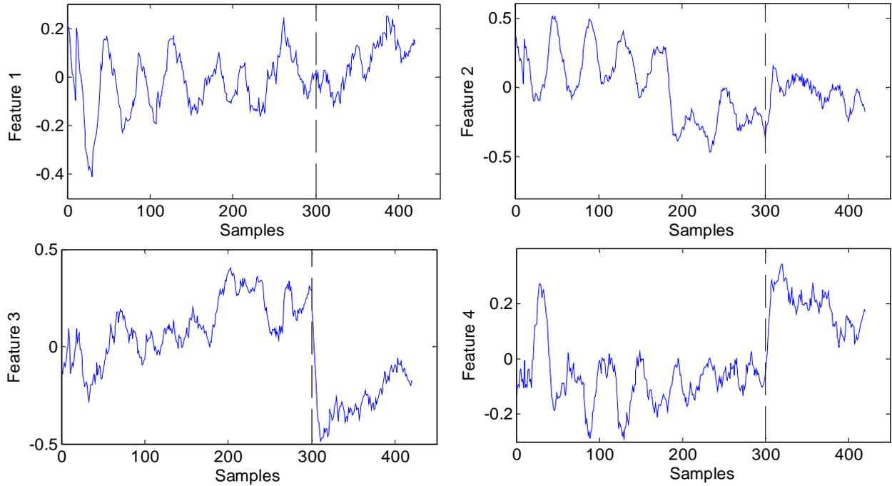
Figure 11: Damage features after reduced order realization through SVD: damage occurrence identifiable at the 300<sup>th</sup> observation as trend discontinuity.
