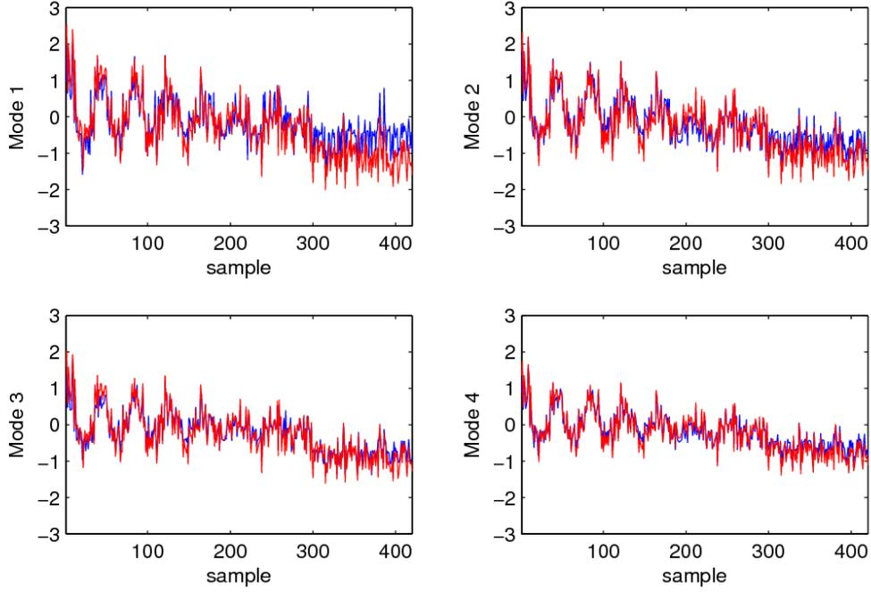
Figure 7: Evolution of  $\frac{\Delta f_n}{f_n}$  (blue curve) and of  $v_n \frac{\Delta T}{T}$  (red curve) throughout the tests carried out on the non-stationary system for the four first modes. Damage is introduced by saw-cut after the 300<sup>th</sup> sample.
