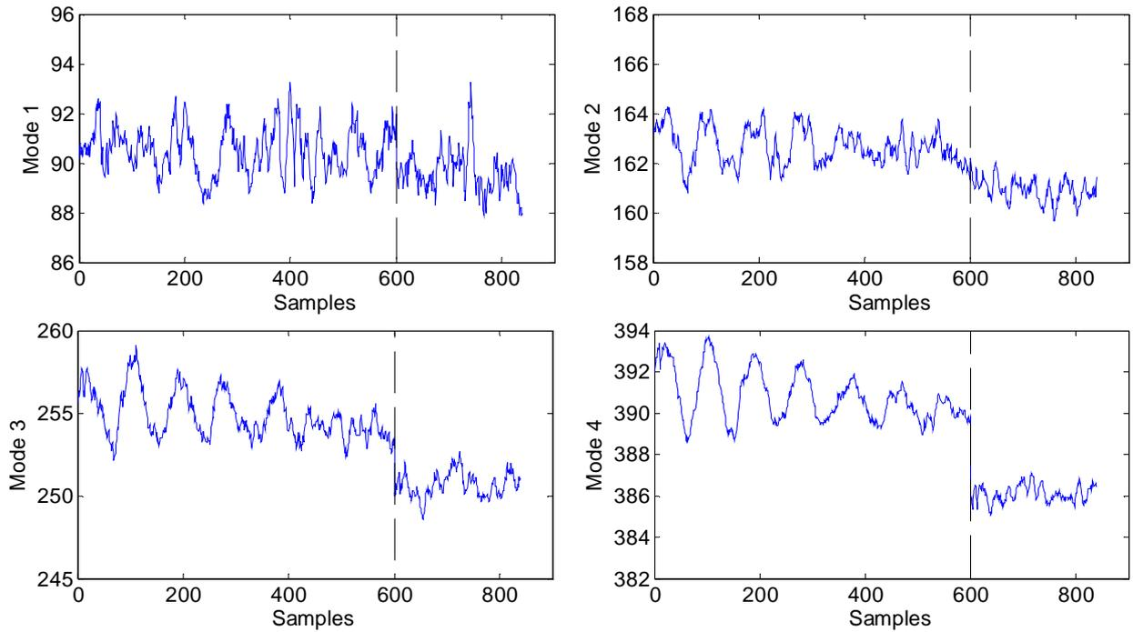
Figure 9: Evolution of the natural frequencies [Hz] throughout the tests carried out on the non-stationary system: damage introduced by saw-cut after the 600<sup>th</sup> sample.
