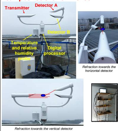
The transmitter generates four parallel laser sheets and the detectors measure the light refracted by the hydrometer (liquid drop) falling through the sampling area:
