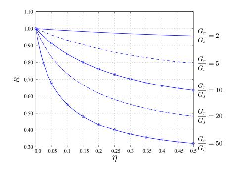
Fig. 11. Risk reduction factor of cross trench configuration as function of  $\eta$  for fixed values of  $\frac{G_r}{G_r}$ .
