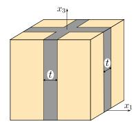
Fig. 7. Unit cell for a cross trench configuration of reinforcement.
