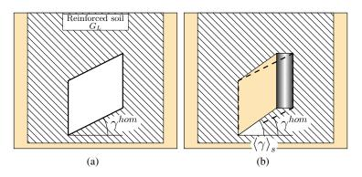
Fig. 3. Shear strain amplitude: (a) case of reinforced soil see as a homogenized material, (b) decomposition in both constituants.
