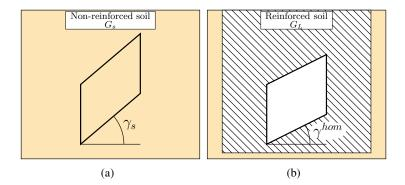
Fig. 2. Shear strain amplitude: (a) case of non-reinforced soil, (b) case of reinforced soil.
