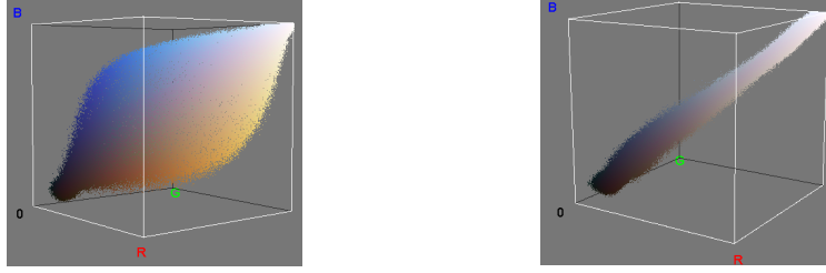
Fig. 7. 3D color clouds of the calibration image before (left) and after (right) correction.
