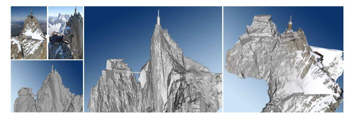
Figure 1. From left to right: two of the 51 images (5 Mpixels) of a mountain summit taken from a helicopter (C B.Vallet/IMAGINE) and the visibility consistent mesh  $M^0$ ; final reconstruction without and with texture remapping using [1] (600, 000 triangles).
