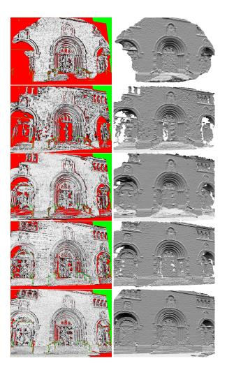
Figure 5. A visual comparison on the *Herz-Jesu-P8* data set. From top to bottom, results from ZAH [51], ST4 [39], TYL [45], FUR [9] and our work. Left: variance weighted depth difference (red pixels encode an error larger than  $3\sigma$ ; green pixels encode missing LIDAR data; the relative error between 0 and  $3\sigma$  is encoded in gray. Right: diffuse renderings of the corresponding triangle meshes.
