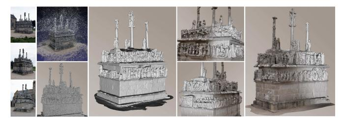
Figure 2. From left to right: three of the 27 images (8 Mpixels) of a sculpted calvary taken from the ground; the generated point cloud (1, 300, 000 points) and visibility consistent mesh  $M^0$  (1, 200, 000 triangles); final reconstruction (1, 850, 000 triangles); close views of the final reconstruction with and without texture remapping. Note the high percentage of outliers in the point cloud and to what extent  $M^0$  is noisy but close to the solution in position and topology.
