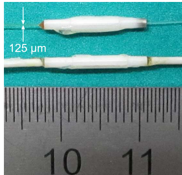
(b) Semi-reflective mirror in ferrule with sheathed and unsheathed optical fiber.
