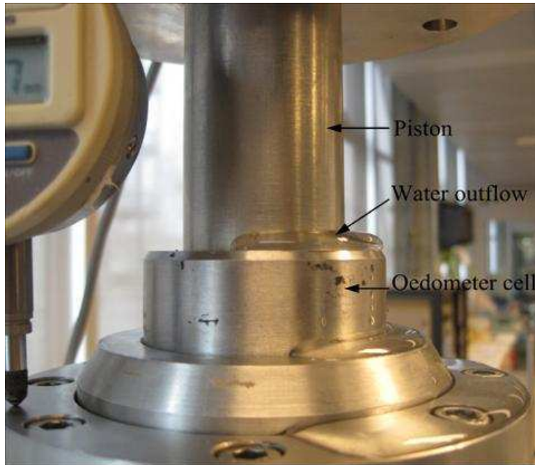
Photo 1. Water outflow through the technological void.
