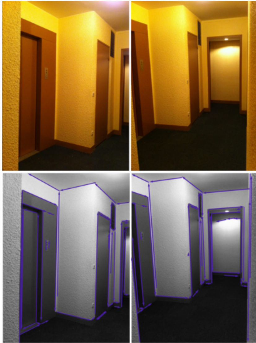
Fig. 9. Second sequence. Top: Original images. Bottom: Detected segments after fragments removal.
