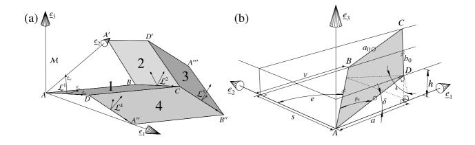
Figure 2: The four elementary faces of the pattern (a) and Face 1 orientation (b).
