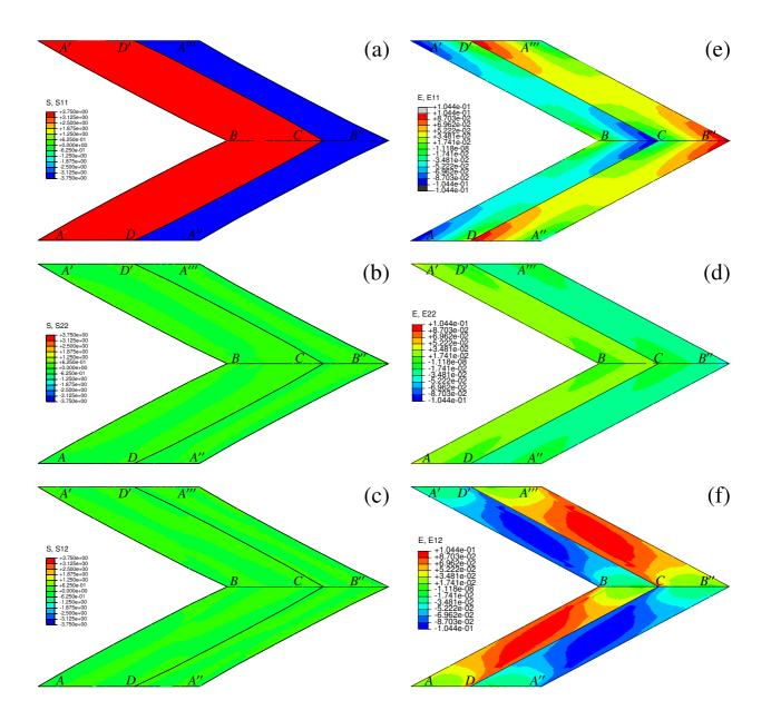
Figure 8: Membrane stresses for  $\tau_1$  load,  $\delta = 72^\circ$ ,  $\zeta = 34^\circ$  ((a):  $\sigma_{uu}$ , (b):  $\sigma_{vv}$ , (c):  $\sigma_{uv}$ ) and membrane strains for  $\gamma_1$  load,  $\delta = 72^\circ$ ,  $\zeta = 34^\circ$  ((d):  $\varepsilon_{uu}$ , (e):  $\varepsilon_{vv}$ , (f):  $\varepsilon_{uv}$ )
