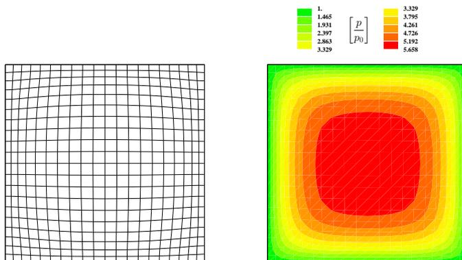
Figure 13: Typical deformed mesh and pore pressure field.
