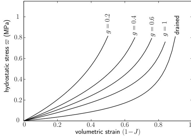
Figure 4: Undrained hydrostatic compression for different values of the fluid parameter  $g$ .
