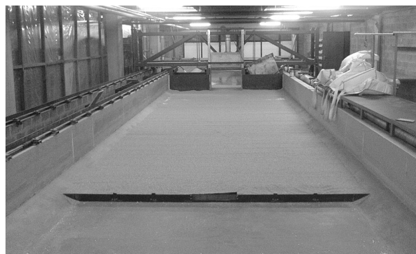
Figure 3. General view of the flume with the initial sand layer (view from downstream)
