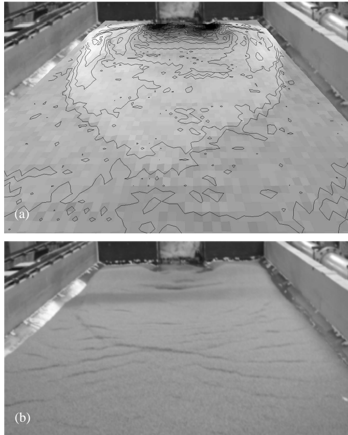
Figure 8. Final bed topography for Case 1: (a) perspective view from downstream, reconstructed from the measured bed profiles and (b) photograph taken after removing the water at the end of the experiment.
