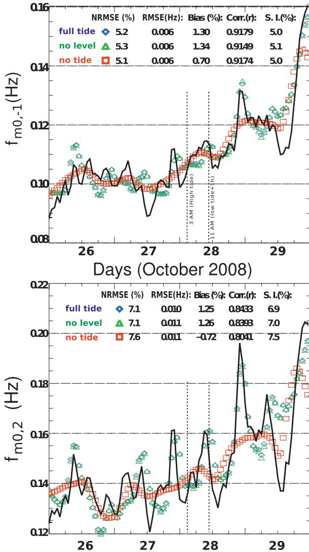
FIG. 10. Mean frequencies (a)  $f_{m0,-1}$  and  $f_{m0,2}$  modeled (symbols) and measured (solid line) at the buoy 62069 in October 2008. Model results are shown, taking into account both water levels and currents (full tide), only the currents (no level), or no tidal effects at all (no tide). The vertical dashed lines mark the 0300 and 1100 UTC (high tide and low tide + 1 h) times that corresponds to the maps shown in Fig. 9.
