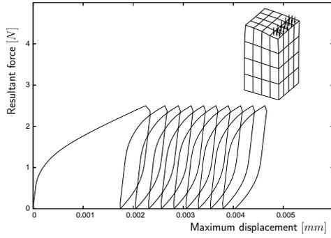
**Fig. 4** Non-homogeneous cyclic loading of amplitude  $400\text{ KPa}$  and period  $T = 40\text{ s}$ .
