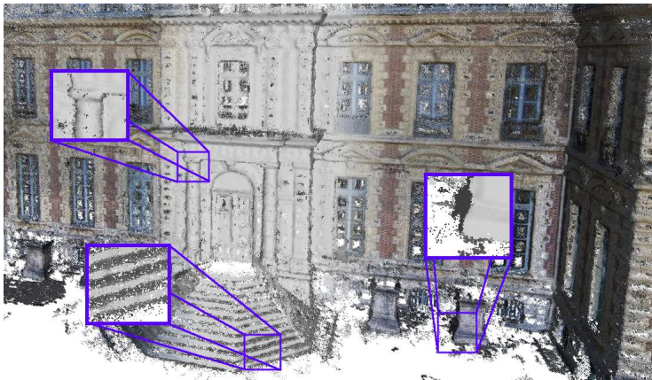
Point cloud created by photogrammetry.
