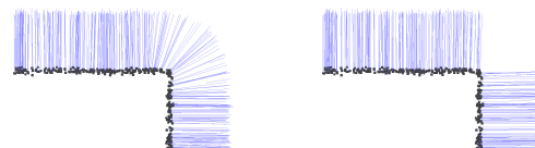
Figure 1: Reconstructed normals of a corner with Least Square Regression (left) and our method (right).
