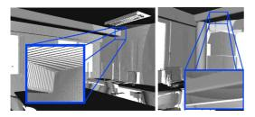
Figure 2: Laser scan of room, highlights of a corner with density anisotropy and a beveled edge.
