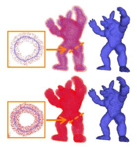
Armadillo with 0.2% noise and +100% outliers (top), +300% (bottom). Neighborhood radius r is 3% of bounding box diagonal. Outliers are uniformly drawn at distance at most r from original point set. Outliers are dropped in result for visual rending (right).
