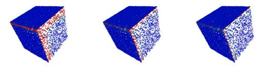
From left to right: RRHT\_Points\_c, RRHT\_Cubes\_c and RRHT\_Unif\_c. Color scale: blue to green is 0 to 10-degree error, red corresponds to an error greater than 10 degrees. Density is uniform on each face; if density is 1 on right face, then it is 5 for the left face and 10 for the upper face.
