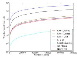
Computation time for a point cloud on sphere with 0.2% noise as a function of the number of points.
