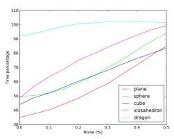
Ratio of the execution time with and without the confidence interval criterion as a function of noise level. **Figure 7:** *Impact of the confidence interval criterion.*
