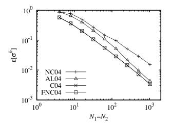
Figure 5: relative error (40) on the stresses for the problem sketched on figure 2, with  $\mu_i = 0$ ,  $\mu_0 = 1.0$  and  $\nu_0 = 0.3$ . NC04: non-consistent scheme; AL04: augmented Lagrangian scheme [16]; C04: consistent scheme; FNC04: filtered, non-consistent scheme.
