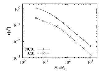
Figure 3: relative error (39) on the polarization for the problem sketched on figure 2, with  $\mu_i = 0.01$ ,  $\nu_i = 0.3$ . NC01: non-consistent scheme,  $\mu_0 = 1.0$ ,  $\nu_0 = 0.3$ ; C01: consistent scheme,  $\mu_0 = 1.0$ ,  $\nu_0 = 0.3$ .
