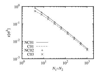
Figure 4: relative error (40) on the stresses for the problem sketched on figure 2, with  $\mu_i = 0.01$ ,  $\nu_i = 0.3$ . NC01: non-consistent scheme,  $\mu_0 = 1.0$ ,  $\nu_0 = 0.3$ ; C01: consistent scheme,  $\mu_0 = 1.0$ ,  $\nu_0 = 0.3$ ; NC02: non-consistent scheme,  $\mu_0 = 0.001$ ,  $\nu_0 = 0.3$ ; C03: consistent scheme,  $\mu_0 = 0.5$ ,  $\nu_0 = 0.3$ .
