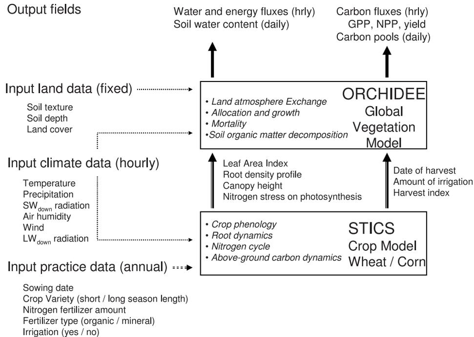
**Figure 1.** Coupling of the ORCHIDEE dynamic global vegetation model with the STICS crop model. Dotted line indicates the gridded input fields which are common to both models. Double dotted arrows indicate input practice data (uniform over Europe). Double solid arrows indicate the variables which are sequentially assimilated from STICS into ORCHIDEE each day. Thick solid arrows indicate the output fields.
