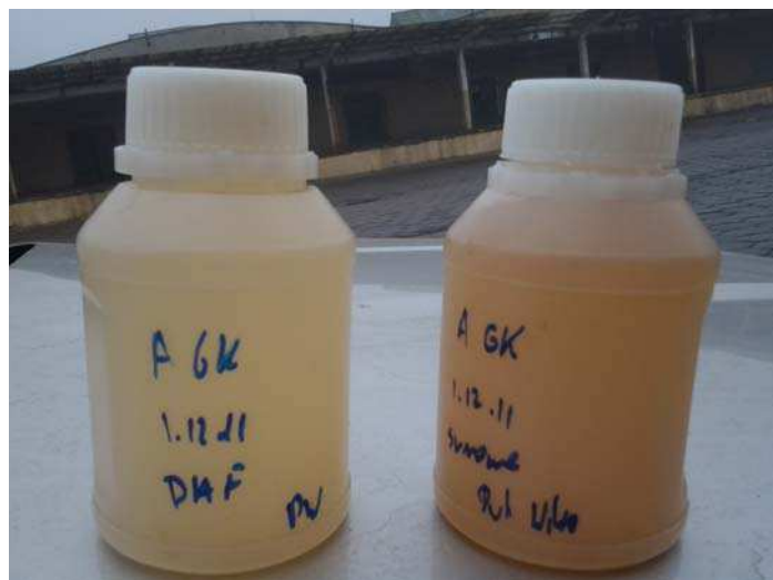
Figure 2: DAF effluent and raw wastewater during tests
