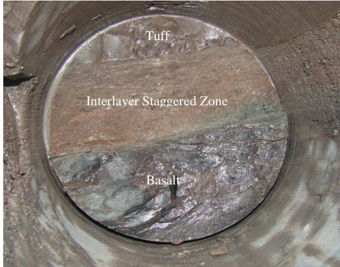
Fig.2. *Interlayer staggered zone in testing tunnel No.62.*
