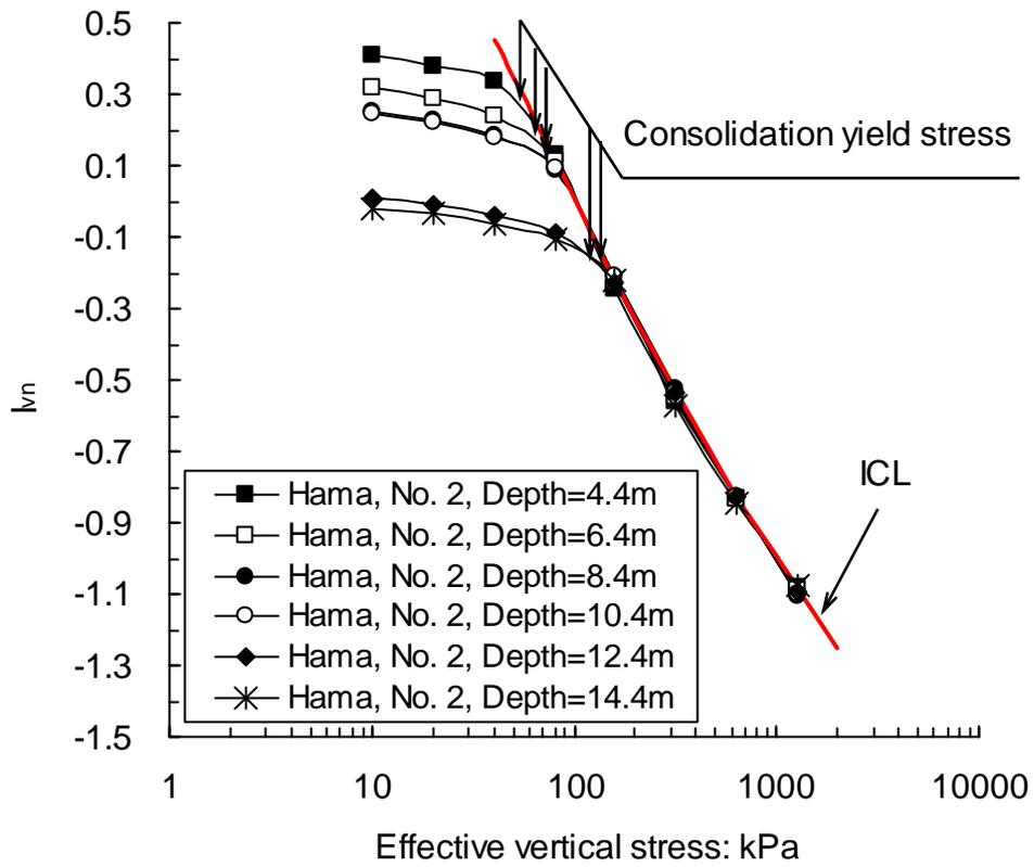
Fig. 15. Typical normalized behaviour of natural Ariake clays with void index  $I_{vn}$
