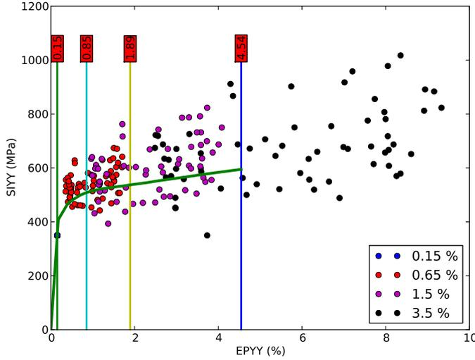
**Fig. 7** Microscopic strain-stress relationship for various nodes within Grain #24 and mean tensile curve
