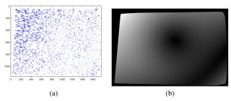
**Fig. 4**: (a) The (subsampled) distortion field directly defined on "inlier" correspondences after the loop validation. (b) Modulus of the dense distortion field obtained by affine interpolation.
