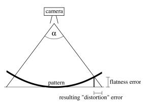
**Fig. 7**: A flatness error in the pattern can be mistaken for a "distortion". In the experiments, with  $\alpha \approx 65^{\circ}$  and a flatness error about 100  $\mu$ m, the produced "distortion" error is about 64  $\mu$ m (flatness error  $\times \tan \frac{\alpha}{2}$ ). Our pattern has the size 406  $\times$  271 mm and produces a 1761  $\times$  1174 image, then one pixel corresponds to 230  $\mu$ m. Thus the observed error would be approximately 0.3 pixel.
