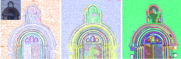
Figure 3. Mesh segmentation using [24]. From left to right: one of the input images and results from approximated mesh based surfaces with various levels of density. Each cluster is drawn with some random color. (NB: on the right column, triangles are so small that the mesh seems plain)
