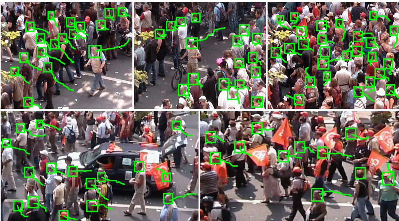
Figure 8. Examples of detection and tracking results for different crowded scenes and levels of person density. For detection (top), true positives are shown in green, false positives are shown in red. The additional true positives detected by the proposed density-aware detector (compared to the baseline with geometric filtering and tracking) are shown in yellow. False positives removed by the proposed method are shown by red dashed line. For tracking results (bottom), head detections are depicted with green bounding boxes along with their associated tracks over 100 frames. Additional results and videos are available on the project web page [1].
