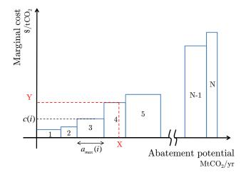
Figure 1: A measure-explicit MAC curve exhibits abatements options 1..N characterized by their maximum potential  $a_{max}$  and their abatement cost c, ranked from the least to the most expensive. This curves stands for a given date in the future T. We find, maybe counter-intuitively, that the optimal mitigation strategy to reach a short-term target X is not to implement exclusively the measures cheaper than Y.
