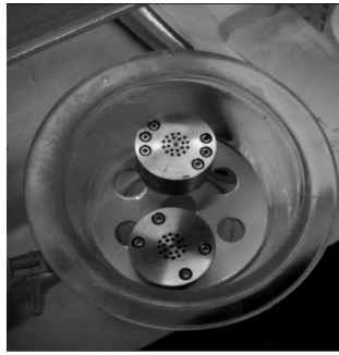
Fig. 2. Constant-volume hydration cell
